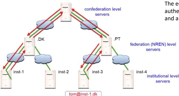
The eduroam service uses IEEE 802.1X as the authentication method and a hierarchical system of RADIUS servers
